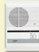
LE-BN Audio Only Privacy Sub Station • Semi-flush mount • Privacy button 8-1/4" H 6" W 2" D (9/16" goes inside wall)
