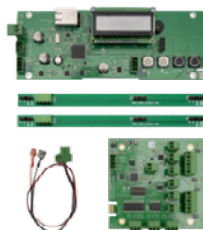
ACS-2DR Two-Door Access Control Starter Kit (includes one door master controller, one AC-2DE expander board, and two AC-STRIPs—included with ACS-2DR-C kit and is sold separately for AC-CA1 enclosure, p. 13)
