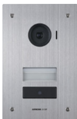
JV-DVF Video Door Station (included with JVS-1F box set—not sold separately)
